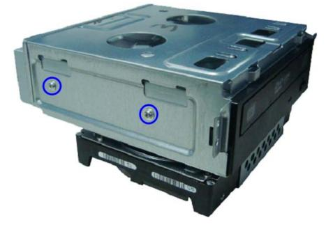
6. Pull the optical drive out of the drive bay.
